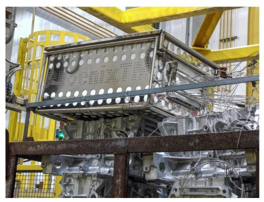
Fig. 3. A PhoenixTM thru-process temperature profiling system is installed in the product cage monitoring the T6 heat treatment (solutionizing, quench and age hardening) of aluminum engine blocks.
