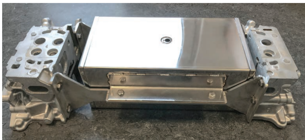
Prepared Aluminium part fitted with the PhoenixTM profile system
