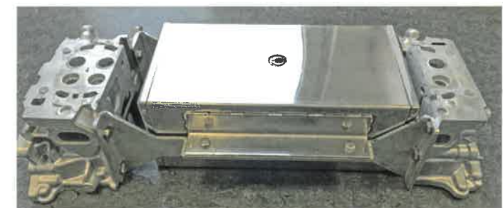
Fig. 4: Prepared aluminium part fitted with the PhoenixTM profile system
