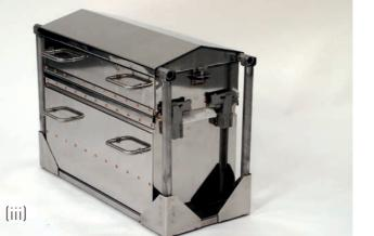
Figure 3. Thermal Barrier Designed Specifically for LPC with Gas Quench.
