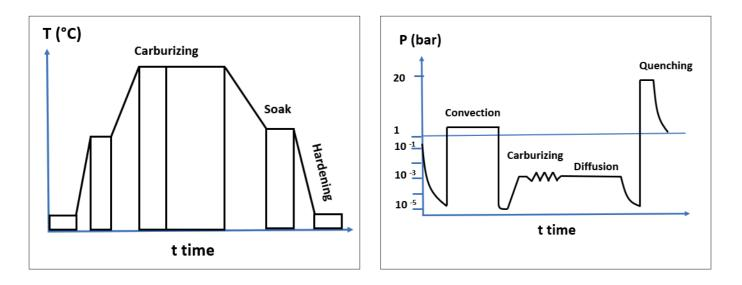
Figure 1. Schematics of the LPC Carburizing process showing the Temperature and Pressure steps
