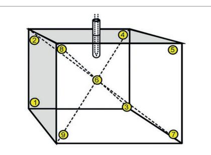
Figure 7. Typical TUS thermocouple Positions - 9 Point Survey. Furnace void corners and center.
