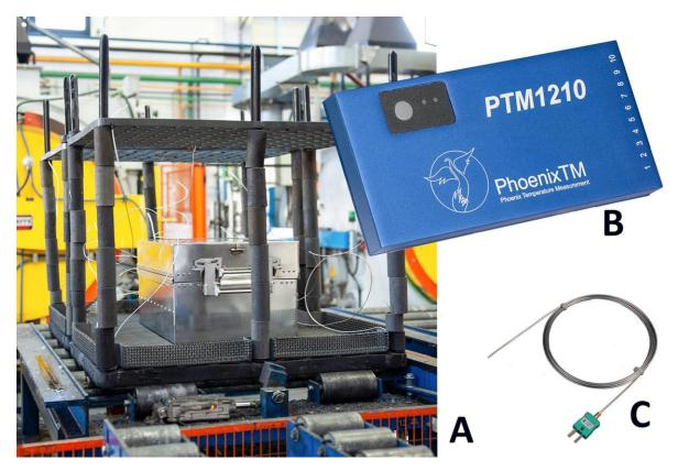
Fig. 2. The PhoenixTM thru-process TUS system is installed in a TUS frame, allowing independent travel through the furnace. The thermal barrier (A) protects the internal multi-channel data logger (B). Short, nonexpendable mineral-insulated thermocouples (C) measure temperature over the qualified work zone.
