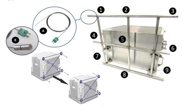
Fig. 4. The PhoenixTM thru-process TUS system shows a TUS frame for use applying the plane method. Thermocouples are installed at nine locations either with (A) an exposed hot junction or (B) a heat sink.
