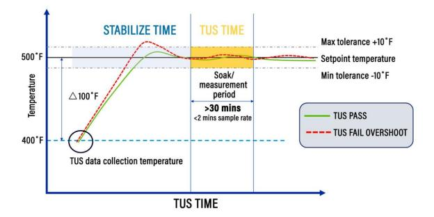
Fig. 1. Schematic of typical TUS result using hypothetical AMS2750G parameters. The green trace is a pass, while the red trace is a fail due to overshoot.
