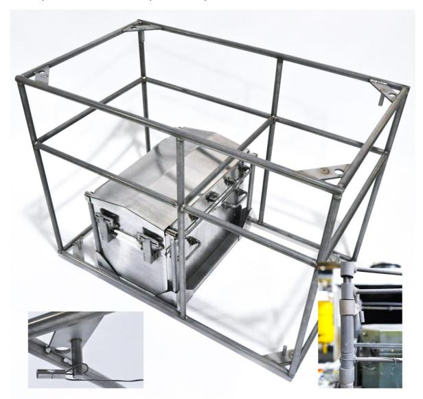
Fig. 3. This PhoenixTM thru-process TUS system is installed in a volumetric TUS frame. Thermocouples are mounted on fixed mounts at the eight vertices of the frame and center point as shown with heat sink fixed to the sensor hot junction.
