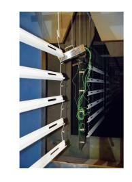
Fig 1. PhoenixTM Compact System travelling through a Powder Coating Oven monitoring Aluminium Extrusions
