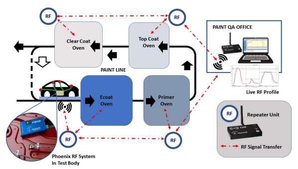
PhoenixTM Thru-process Monitoring in Automotive Coating
