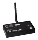
Fig 7: PhoenixTM Remote repeater used to transfer RF signal back from Ovens to monitoring PC
