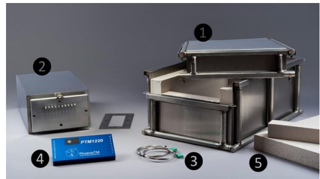
Fig. 5 - ‘Thru-process’ temperature monitoring system oil quench compatible thermal barrier design.
