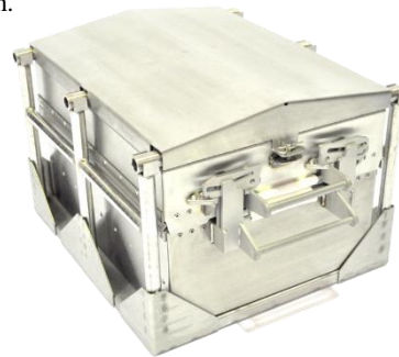
Fig. 7 - Thermal barrier designed for protecting the data logger against severe temperature and pressure changes in the LPC N 2 / Helium Gas quench at 20 bar pressure. Quench deflector shown fitted to barrier.
