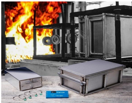
Fig. 1 - Thru-process temperature profiling system shown entering a gas carburising furnace, heat treating automotive gears. The data logger travels through the Furnace, protected by a thermal barrier, with the product being monitored collecting a thermal profile of the heat treatment process.
