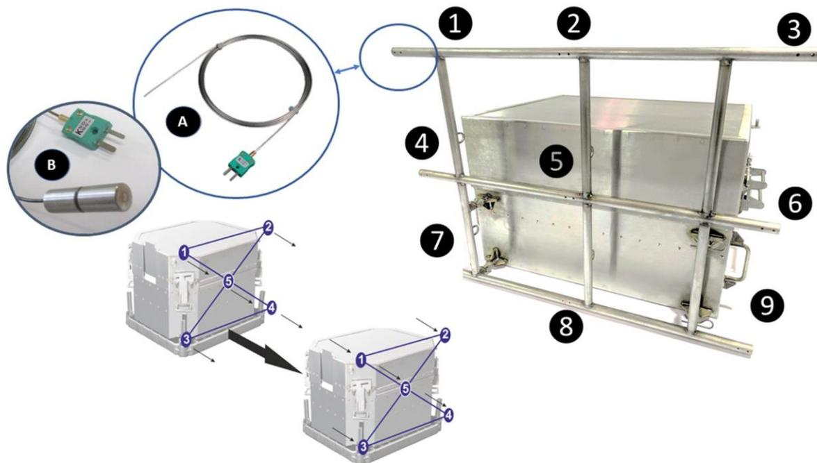
**Fig. 4. The Phoenix™ thru-process TUS system shows a TUS frame for use applying the plane method. Thermocouples are installed at nine locations either with (A) an exposed hot junction or (B) a heat sink.**
