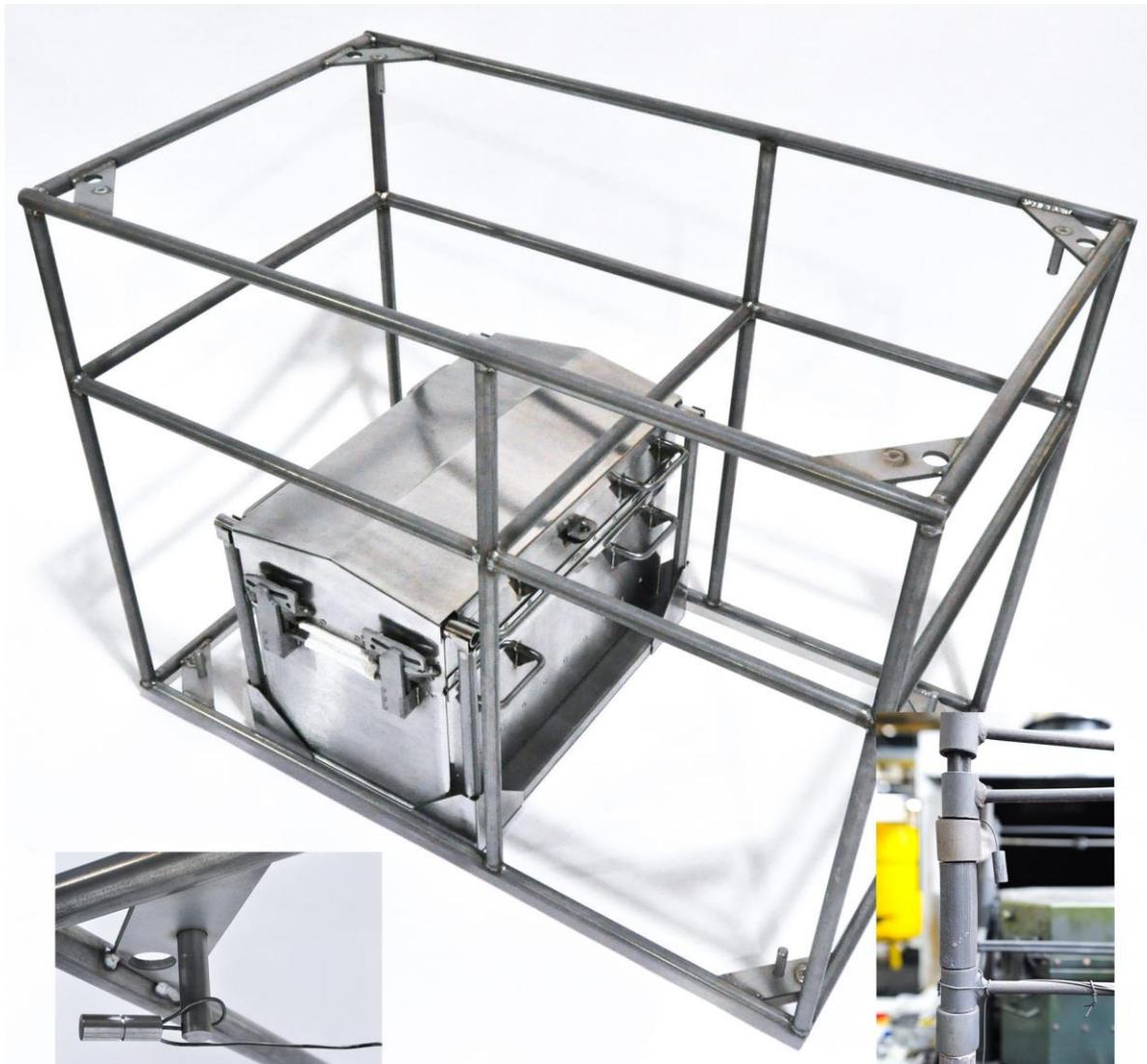
**Fig. 3. This Phoenix™ thru-process TUS system is installed in a volumetric TUS frame. Thermocouples are mounted on fixed mounts at the eight vertices of the frame and center point as shown with heat sink fixed to the sensor hot junction.**
