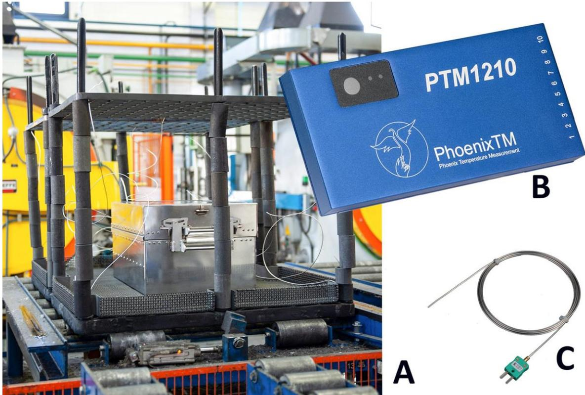
**Fig. 2. The Phoenix<sup>TM</sup> thru-process TUS system is installed in a TUS frame, allowing independent travel through the furnace. The thermal barrier (A) protects the internal multi-channel data logger (B). Short, nonexpendable mineral-insulated thermocouples (C) measure temperature over the qualified work zone.**
