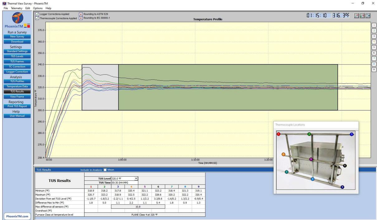
**Fig. 5. PhoenixTM Thermal View Survey software shows the visual and data analysis of a specific TUS level using the plane method applied to a continuous belt furnace.**
