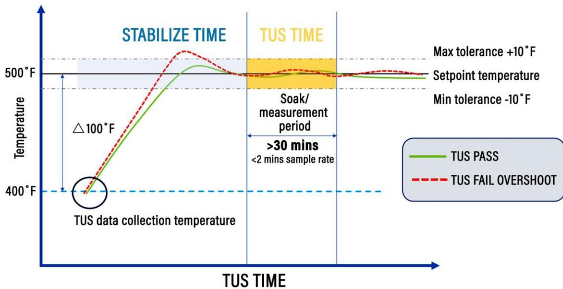
**Fig. 1. Schematic of typical TUS result using hypothetical AMS2750G parameters. The green trace is a pass, while the red trace is a fail due to overshoot.**
