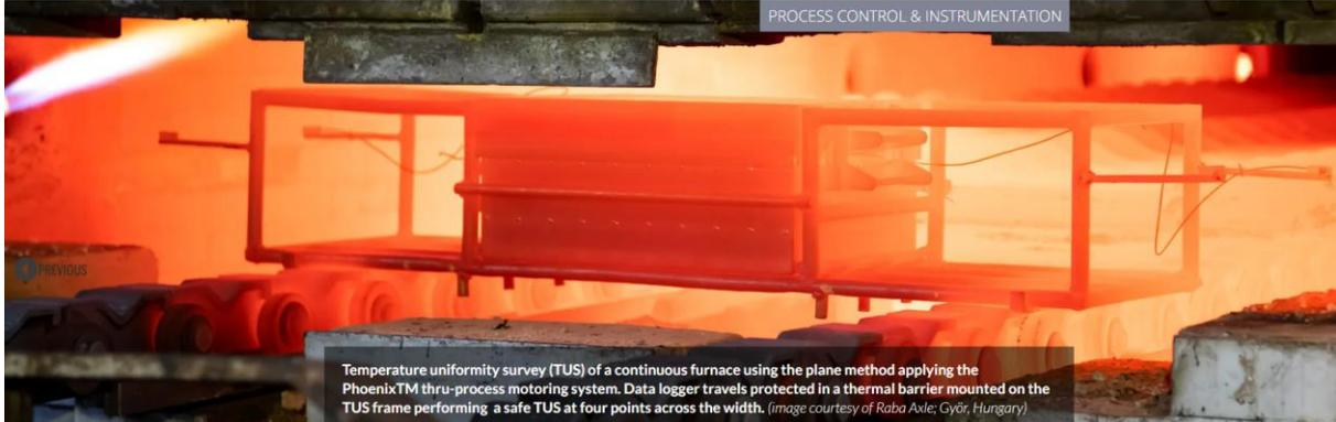
Temperature uniformity survey (TUS) of a continuous furnace using the plane method applying the Phoenix™ thru-process motoring system. Data logger travels protected in a thermal barrier mounted on the TUS frame performing a safe TUS at four points across the width. (image courtesy of Raba Axle, Győr, Hungary)
