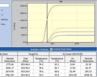
(Tref 70 °C, Dt 16.2 s and Z value 7.5 °C) can be input to calculate for each monitoring point the number of decimal reductions of the pathogen achieved during cook to meet CCP limits.
