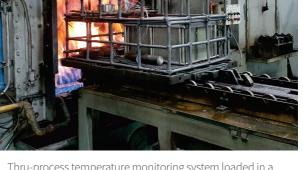
Thru-process temperature monitoring system loaded in a product basket traveling into and through a continuous sealed gas carburizing furnace.
