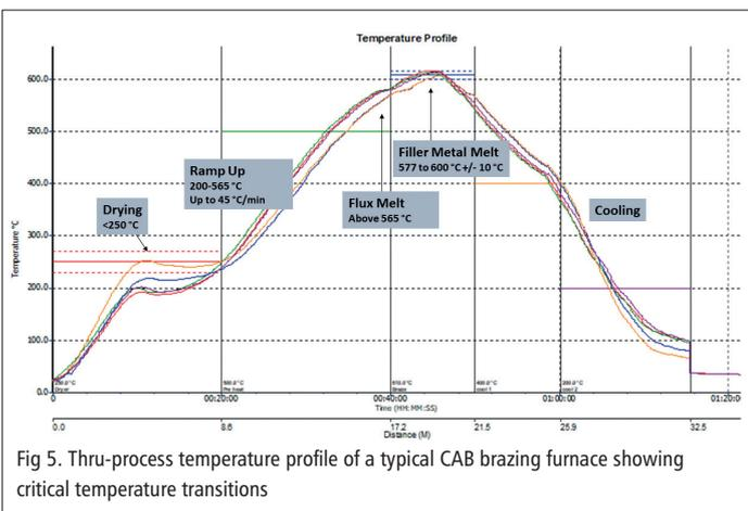
Fig 5. Thru-process temperature profile of a typical CAB brazing furnace showing critical temperature transitions
