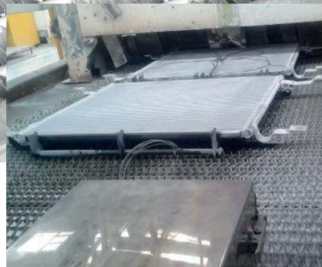
Left: Fig 1. PhoenixTM HTS08 'thru-process' temperature profiling system enters the CAB brazing furnace with product being monitored
