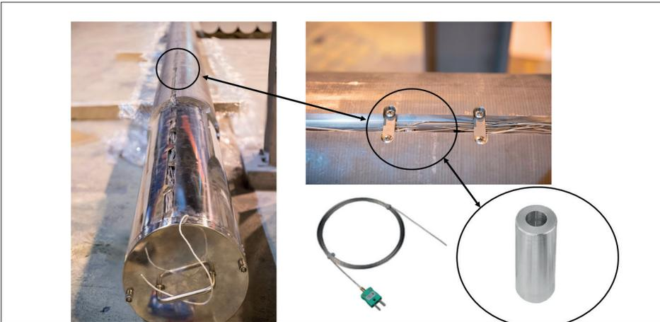
Fig 3. Thermocouple Installation
