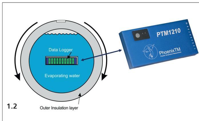
Fig 1. PhoenixTM TS57 Rotating Evaporative Water Barrier solution.
