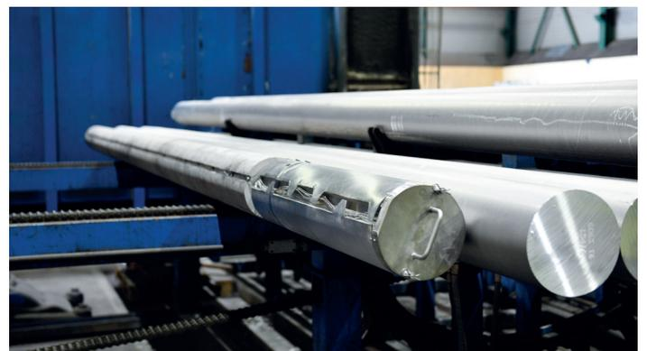
Fig 5. PhoenixTM TS57 Rotating Evaporative Water Barrier Thru-process Monitoring System Set-up at Mäkelä Alu Oy
