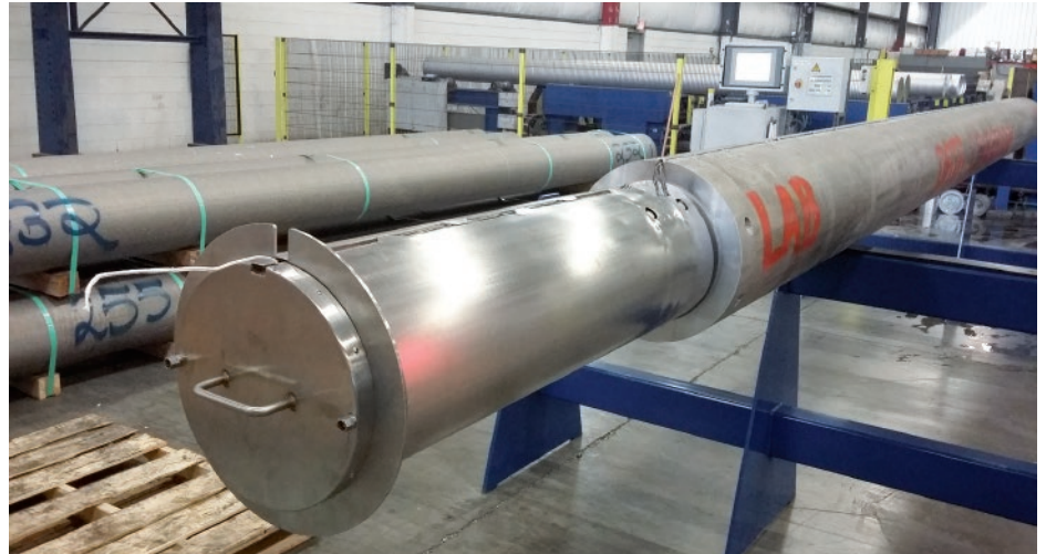
Figure 2. PhoenixTM TS57 Rotating water barrier solution set-up - System is used to successfully routinely monitor in real time the homogenisation of cast aluminium logs in Service Center Metals (SCM) walking beam furnaces. Rotating cylindrical water barrier is attached to a 356 mm / 14" log with thermocouples positioned along its length at varying depths.
