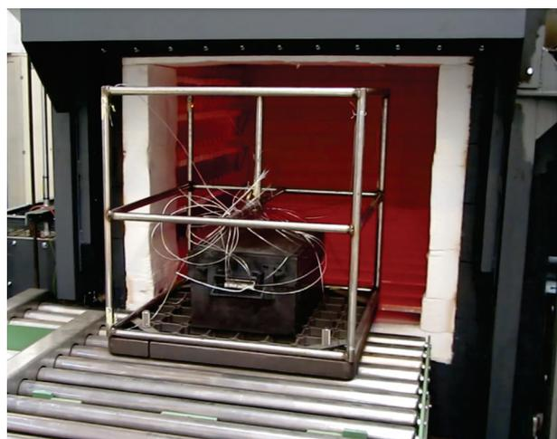
**Fig. 3** — Thru-process temperature monitoring system loaded into a batch furnace with TUS frame to complete a temperature uniformity survey.
