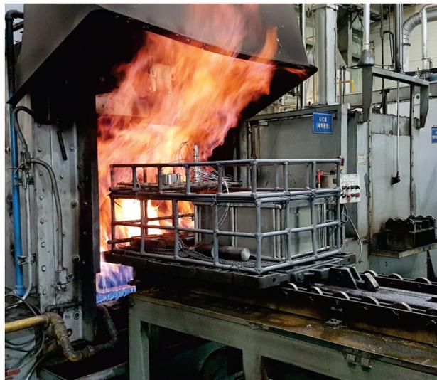
Thru-process temperature monitoring system loaded in a product basket traveling into and through a continuous sealed gas carburizing furnace.
