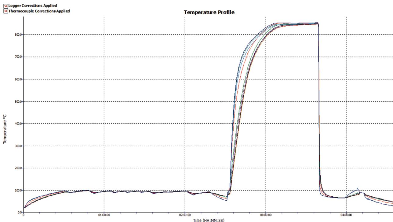
Fig. 1 — Typical thermal profile for thru-process temperature monitoring system through a continuous sealed gas carburizing furnace.
