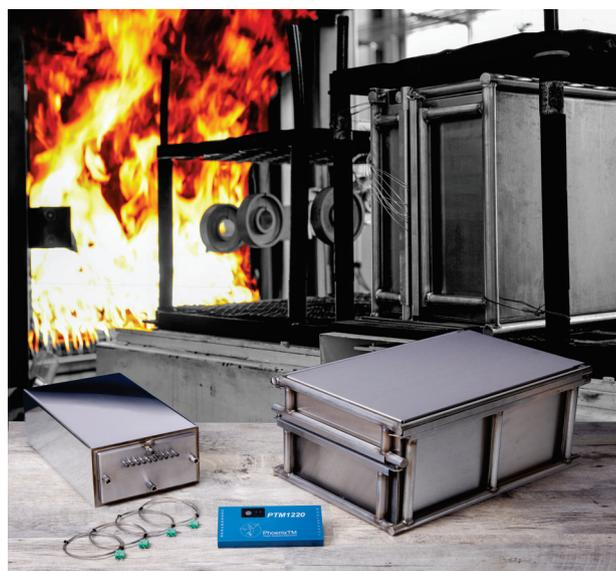
**Fig. 4** — Thru-process temperature monitoring system for use in sealed carburizing furnace with integral oil quench. To the left is the inner sealed thermal barrier and data logger and on the right is the outer structural frame containing sacrificial insulation.
