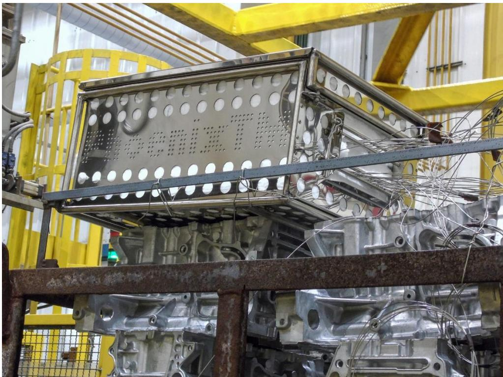
**Fig. 3.** A Phoenix™ thru-process temperature profiling system is installed in the product cage monitoring the T6 heat treatment (solutionizing, quench and age hardening) of aluminum engine blocks.
