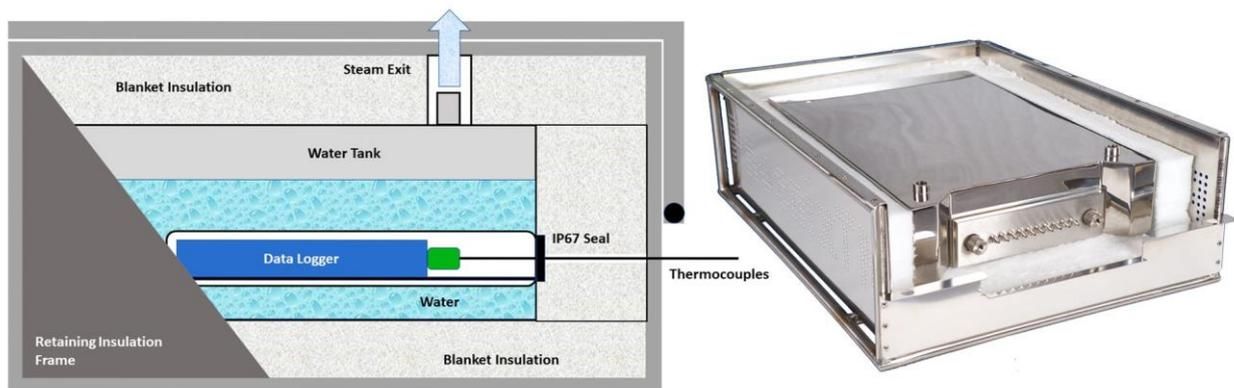
**Fig. 4. TS06 thermal-barrier design is installed within a structural frame containing the insulation blanket surface layer. The water tank is shown with a traditional compression-fitting face-plate seal.**
