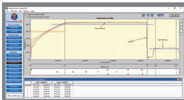
ThermalView Plus Software displaying the full process profile trace
