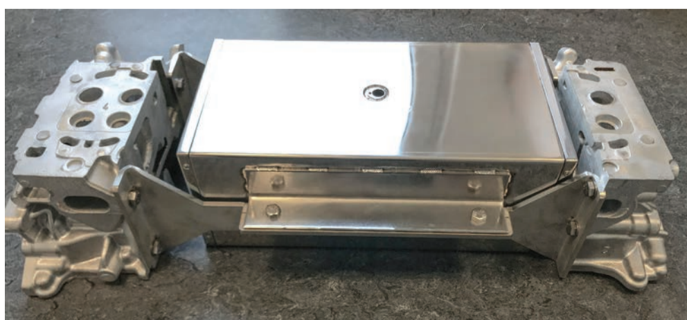
Prepared Aluminium part fitted with the PhoenixTM profile system
