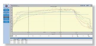
Multiple time above temperature, rates of change of temperature and maximum temperature analysis options for verification of the cure quality and optimisation of the process
