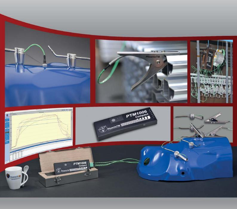
The Compact Finishing System is designed to travel through the curing oven measuring actual product temperatures, providing a low cost durable profiling solution. The system uses a data logger, protected by a thermal barrier, to record the temperature of product as it passes through the oven. Information obtained can then be used to optimise the process.
