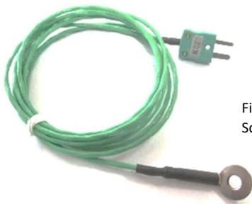
Fig 4: Washer Thermocouple Screwed to test body
