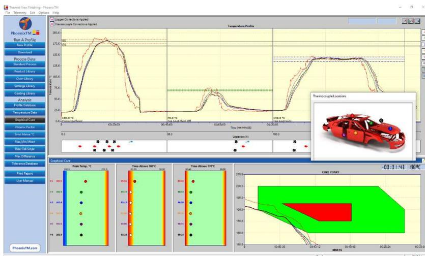
Fig 9: PhoenixTM Thermal View Finishing Software showing the CureChart graphical cure analysis function
