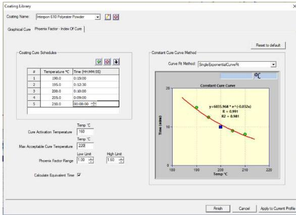
Fig 10: PhoenixTM Thermal View Finishing Software Phoenix Factor – Coating Library file with defined Constant Cure Curve.
