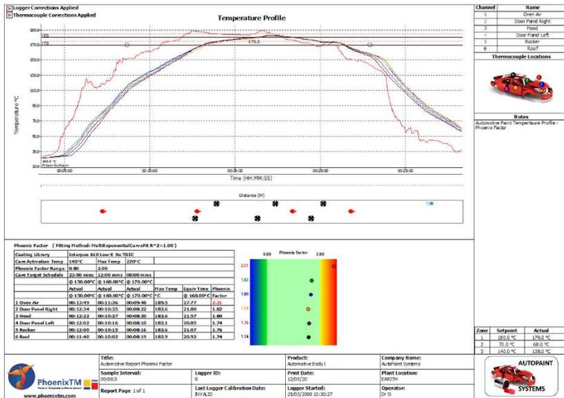
Fig 11: PhoenixTM Thermal View Finishing Software Phoenix Factor – Report and Graphical Pass/Fail Tool.
