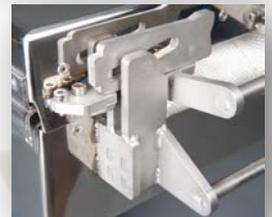
Heat sinks with very high thermal capacity and gas tight seals allow use in vacuum or pressure applications up to 20 bar.
