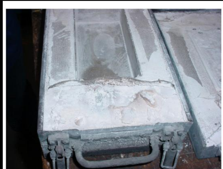
Acid attacks the cloth protecting the insulation
