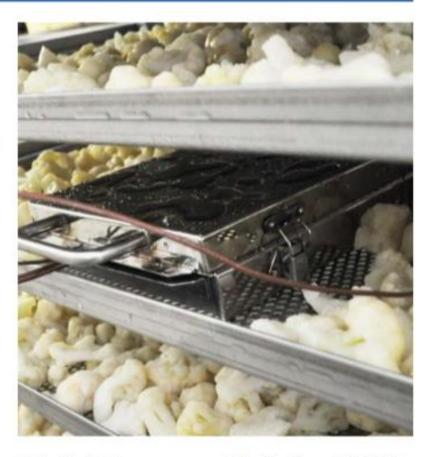
80 °C with a data logger accuracy of ±0.3 °C operating below +50 °C. Data logger and thermocouple correction factors can be further applied to maximise measurement accuracy.
