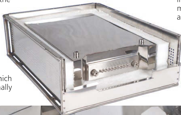
Fig 4. TS06 Thermal barrier design showing water tank, housing the data logger at its core, installed within structural frame containing the insulation blanket surface layer. Water tank shown with traditional compression fitting face plate seal.
