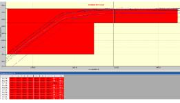
Clear reporting of overshoot errors both graphically and in raw data highlighting exactly where TUS failure occurred.
