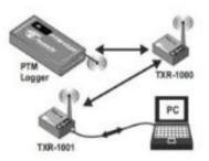
Employing real time operation, product core temperatures over the product rack or conveyor mesh belt width can be monitored live.
