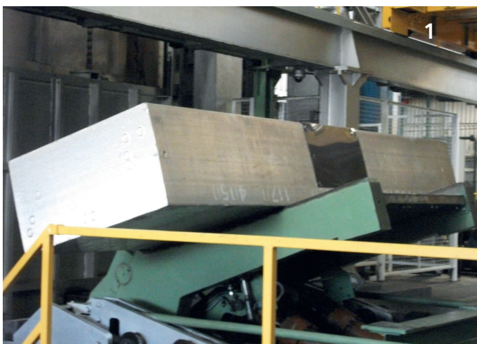
Fig 5. Left and right. Test Slab with installed monitoring system being loaded into the furnace (1) and schematic showing rotation steps (2).
