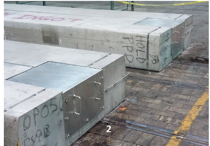
Fig 3. PhoenixTM System embedded in aluminium slab/Ingot (1) - stainless steel cover to protect from high velocity air flow in furnace (2)
