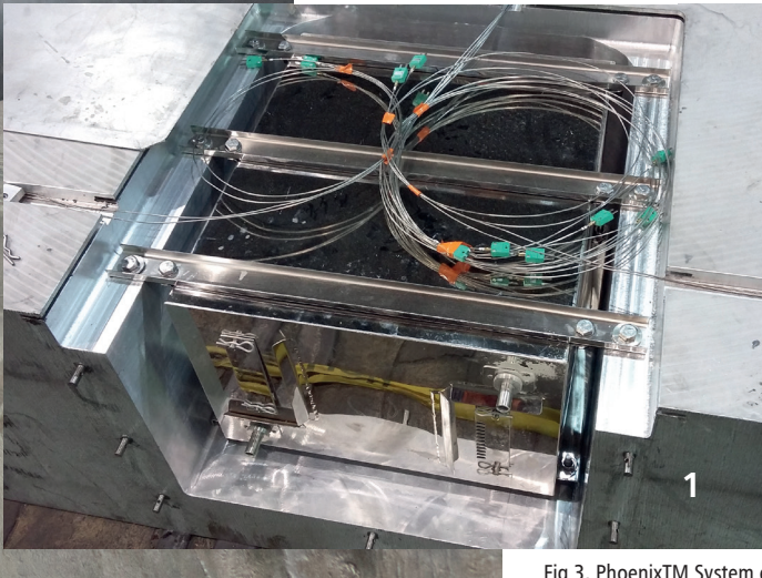
Fig 3. PhoenixTM System embedded in aluminium slab/Ingot (1) - stainless steel cover to protect from high velocity air flow in furnace (2)
