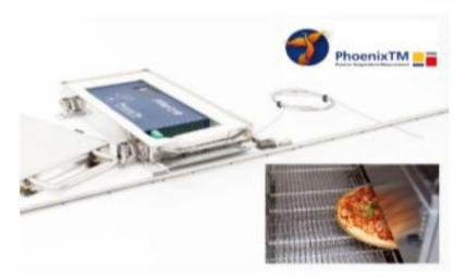
(MI) design operating up to 500 °C (Type K). The MI thermocouples can be inserted into the pizza. Alternatively, to thermally map the oven, thermocouples can be positioned across the belt using the probe jig accessory (Shown above).
