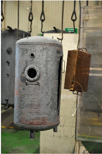
Figure 1: 'Thru-process' temperature profiling system entering a continuous porcelain enamel firing furnace. The thermal barrier protecting the operational data logger travels along with product test piece (boiler tank) being monitored, hung from the overhead conveyor. Short thermocouples attached, to key parts of the product, record temperature during the journey at specified intervals recording the accurate temperature of the product/enamel surface interface.
