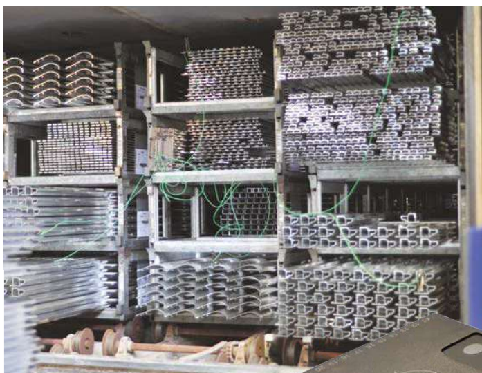
Fig 1. Typical aluminium extrusion ageing oven loaded with separate racks housing different profiles. Phoenix™ system positioned on middle rack with thermocouples running to different key positions in the oven.
