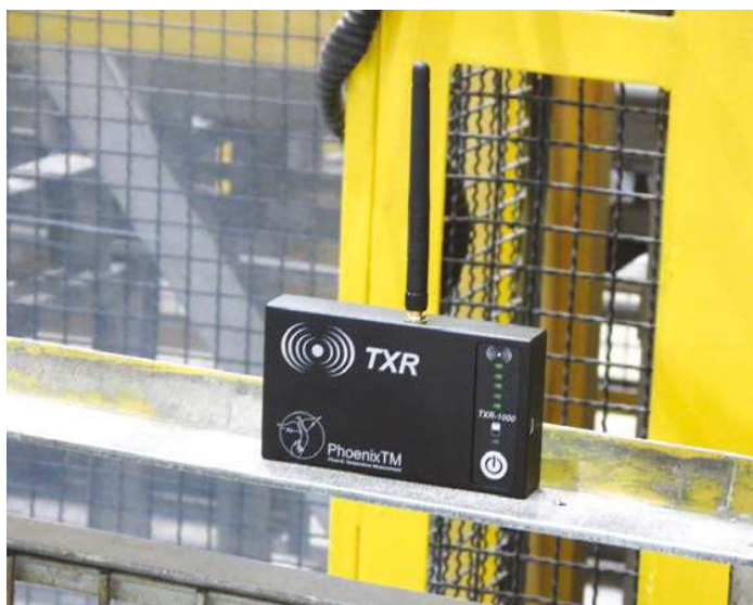
Fig 5. RF Telemetry Repeater transferring the live RF signal from the oven to the monitoring PC.
