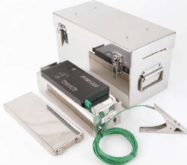
Fig 2. Phoenix™ Thru-process Temperature Monitoring System
