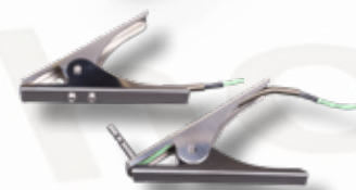
Clamp Probes (TC52/TC53) General paint powder applications where product is non ferrous (eg: Aluminium extrusion). Available for surface or air measurement.
